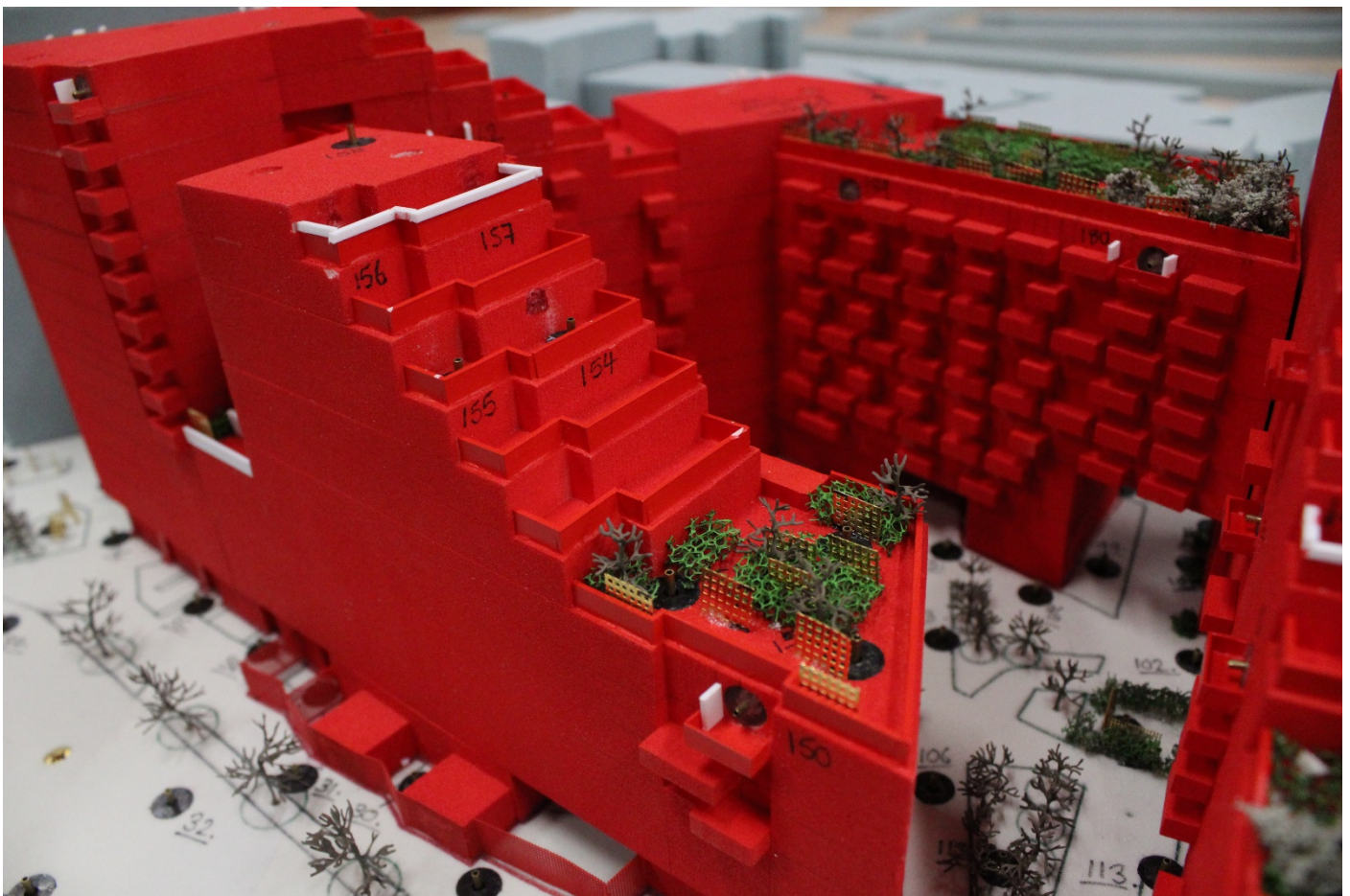
Wind Tunnel Study Model Configuration 4: Proposed Development with existing surrounding buildings and mitigation measures
